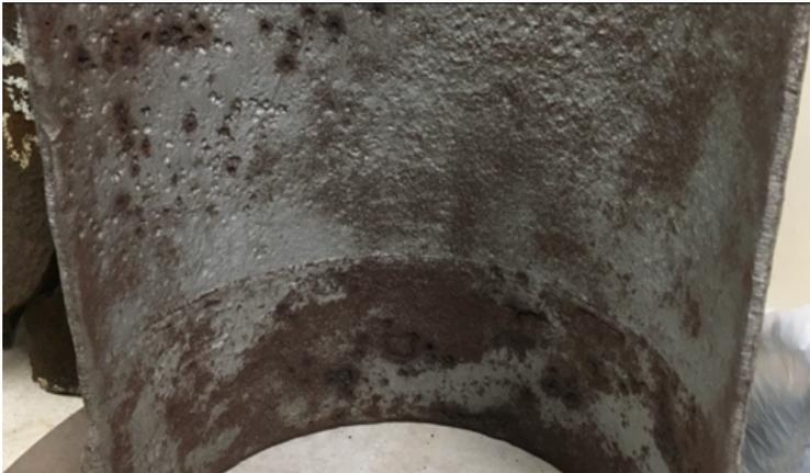
**Figure 1: Precise models and sensors are essential for ultrasonic thickness monitoring, capturing complex changes in reflected ultrasound waves caused by pipe interior corrosion.**
