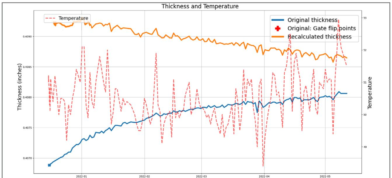
Figure 3: Misleading Thickness Increase Due to Active Corrosion
