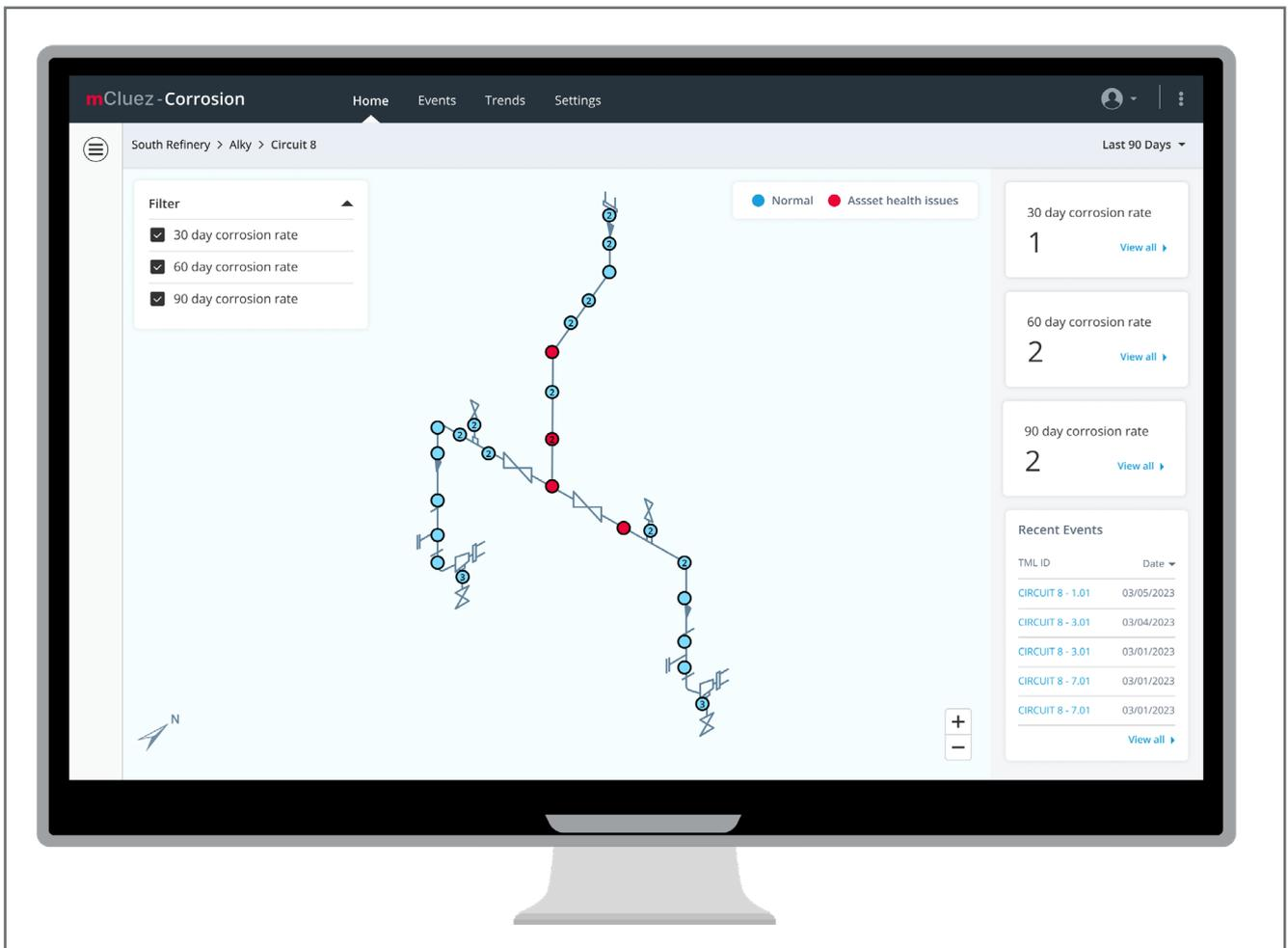
Figure 5: Circuit-Level Visualization of CML Status
