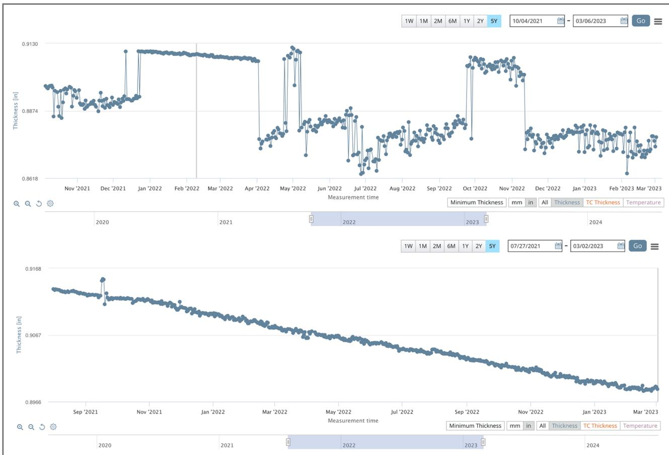
Figure 4: Static Gates vs. Dynamic Gates: A Comparative Study of Thickness Trends
