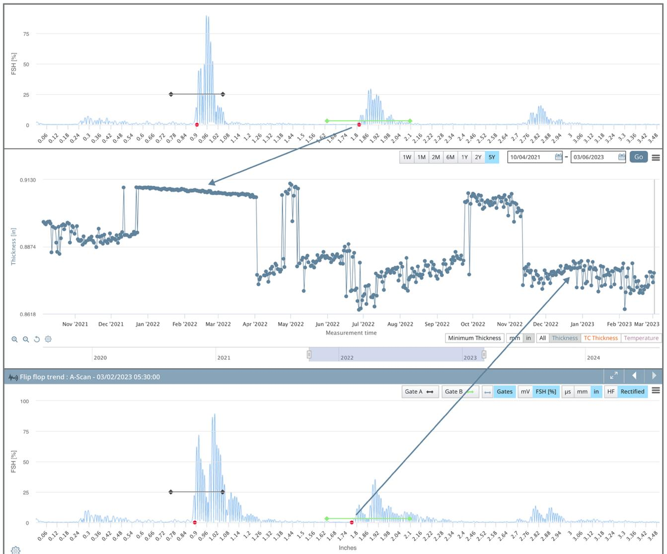
Figure 2: Impact of Corroding Surfaces on Ultrasonic Waveforms and Thickness Measurements
